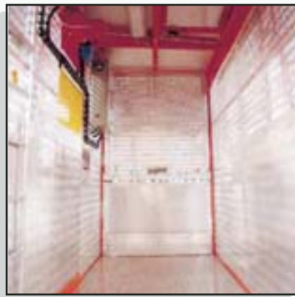
Top-Mounted Machinery for unobstructed cage access
